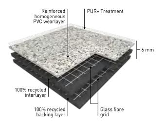
GTI MAX is a multi-layered interlocking looselay vinyl tile with polyurethane treatment (PUR+), 6 mm thick with a dovetail joint for the **CONNECT** configuration and with welded joints for the **CLEANTECH** configuration.
