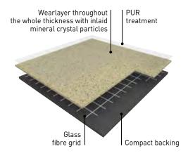
**TARASAFE STANDARD** with **PUR** surface treatment is a slip resistant safety vinyl floorcovering, with a PVC wear layer and deeply inlaid mineral crystal particles (patented). It is reinforced by a glass fibre grid and available in a sheet format. It is an ideal solution for heavy traffic applications where slip resistance, durability, hygiene and easy maintenance are required.
