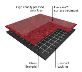
The floor covering is made of a >1mm thick, pure vinyl homogeneous wear layer with no filler, incorporating very densely pressed coloured chips, with a mat finishing and without a transparent wear layer.
