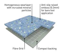
**TARASAFE ULTRA H20** is a slip resistant vinyl floorcovering, with a PVC wear layer and deeply inlaid mineral particles and coloured chips for a decorative design together with a raised emboss for better slip resistance.
