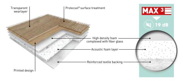
**TARALAY LIBERTEX** is ideal for fast track installation or renovations in commercial buildings. It is a multi-layered vinyl floorcovering with a printed design protected by a 0,70 mm thick transparent wear layer. The product features a high density foam complexed with fiber glass, an acoustic foam layer and a reinforced textile backing. It offers **19 dB sound insulation**.
