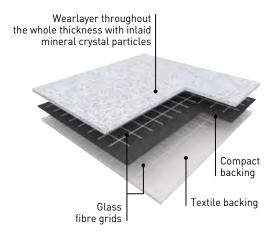
**TARASAFE PLUS** and **TARASAFE SUPER** are slip resistant safety vinyl floorcoverings, with a PVC wear layer and deeply inlaid mineral crystal particles (patented). They are reinforced by a glass fibre grid and available in a sheet format. They are an ideal solution for heavy traffic applications where slip resistance, durability, hygiene and easy maintenance are required.
