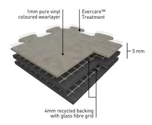
temperature and over 3000 T, a 4mm recycled backing and a 1mm pure vinyl wear layer. This wear layer is incorporating very densely pressed coloured chips, with a mat finishing and without a transparent wear layer. The product comprises a compact backing which is pressed and reinforced with two glass fibre grids.
