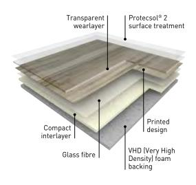
TARALAY IMPRESSION COMFORT 0,65 is an acoustic multi-layered vinyl floorcovering, available in 2m wide sheet, with a group T wear rating. The product comprises a Very High Density (VHD) foam backing reinforced with a glass fibre and a printed design that is protected by a transparent wear layer (0.65 mm thick). It offers 19 dB sound insulation and an indentation resistance of ca. 0.08 mm.
