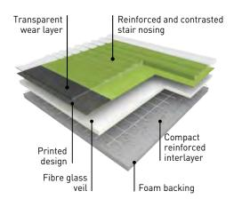
**TARASTEP** is a multilayered and foam backed complete step with a thickness of 3.35 mm. It comprises a printed design, a vinyl transparent wear layer and a specific embossing on stair nosing for safety.
