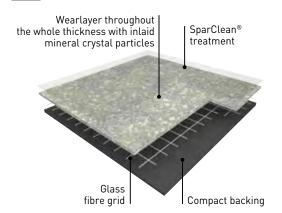
TARASAFE GEO is a slip resistant vinyl floorcovering, with a PVC wear layer and deeply inlaid mineral crystal particles (patented) and coloured chips for a decorative design. It is reinforced with a glass fibre grid in sheet form.
